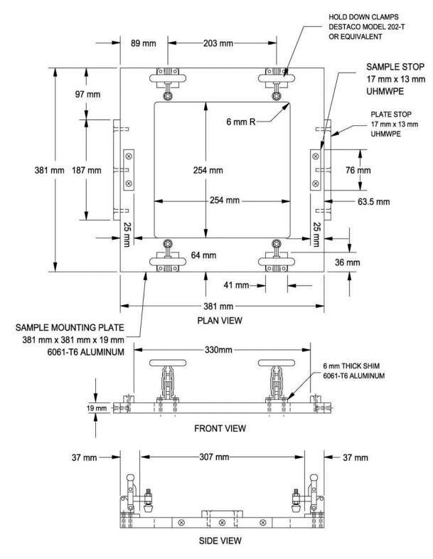
**Figure 4: Sample Clamping Device**
