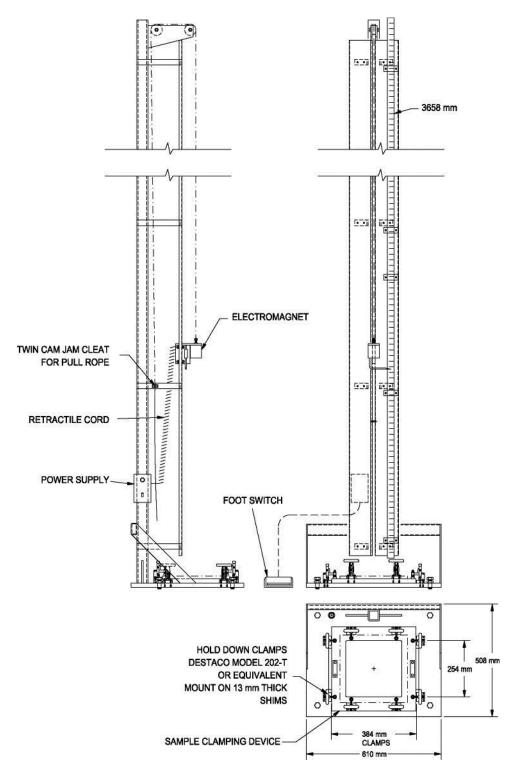
Figure 3: Free Fall Test Stand
